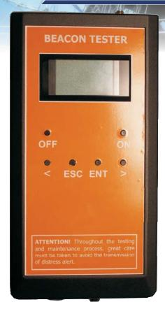
The BEACON Tester is designed to decode and display the encoded message from a 406 MHz Cospas-Sarsat Emergency Position Indicating Radio Beacons. The tester can be connected directly to the EPIRB or monitored "over the air" using the supplied whip antenna. The tester will decode any 406 MHz maritime protocol for EPIRB's.
