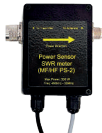
MF/HF Power Sensor & VSWR Meter, PS-2
