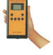
The SART Tester provides measurement of the carrier frequency, duration and power of the response. The device has small dimention and ican be easily placed in hand.
